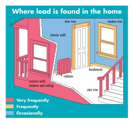
**Look for peeling paint,** especially on window frames and wood trim. Look carefully at the outside of the building, window sills and frames, doors and door frames, and walls in the kitchen and bathroom.
